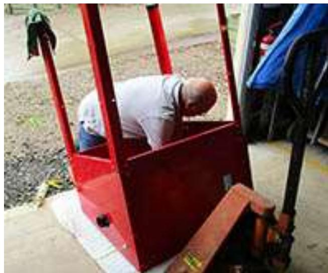
*Graeme Atkins working on a new sand-blasting cabinet in the Metalwork Shed. 27 February 2018.*
